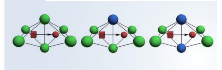
Figure 3: Assumed migration edge configurations in samarium doped ceria. Ce-Ce edge (left), Ce-Sm edge (middle) and Sm-Sm edge (right). Cerium ions (green), samarium ions (blue), oxygen ions (red spheres) and oxygen vacancies (red boxes).
