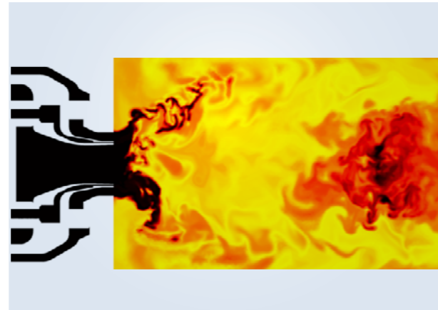
Simulation of combustion and soot formation in a model aeronautic engine
