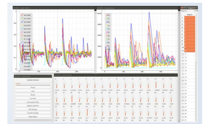
Figure 1: Calcium concentrations and connections are shown for brain regions (top left and right). A region selector allows users to focus on a subset of these (to the right). The steering panels (bottom middle) allow for interactive modification of model parameters while the simulation runs.
